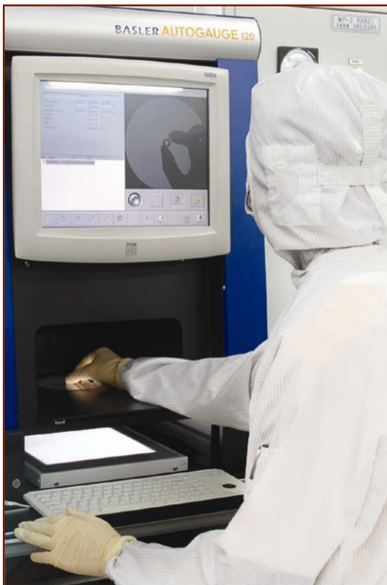
Figure 5. Seal Engineer Verifying Seal Dimensions to Specification
